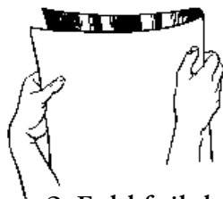
2. Fold foil down length at center but do not crease on the fold.
